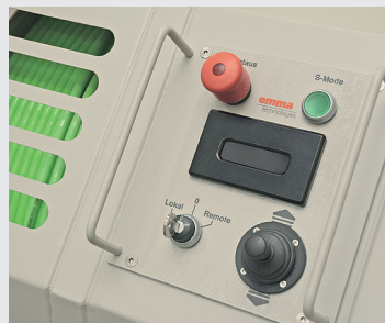
Control panel on the winch
