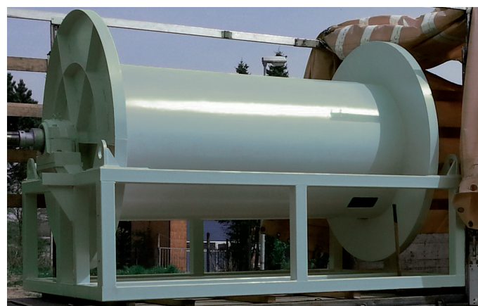
Heavy-Duty Winch for seismic or oceanographic applications
